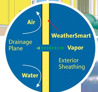
*WeatherSmart protects against water intrusion and air infiltration from the outside, while allowing moisture vapor to escape from the inside.*
